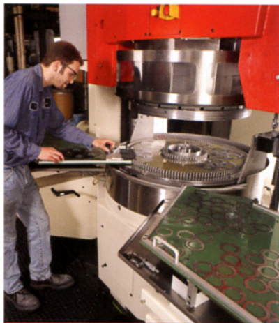
Columbia Grinding uses state-of-the-art flat honing/fine grinding technology to provide ultra-flat finished surfaces on metals, alloys, and other materials. Photos courtesy of Columbia Grinding.
