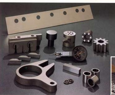
Where toolroom tolerance or special angles are required, Columbia's reciprocating surface grinders are available. These machines are also good on production runs, especially on small or thin pieces (1/4" dia., .013" thick).
